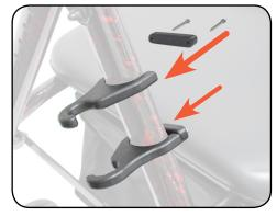
Attach 1 mounting bracket with 2 screws to upper arm and tighten. Repeat for lower arm.
